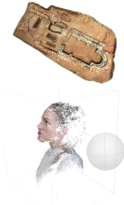
Figure 1. Archaeological site model (a) created from point clouds collected with terrestrial LiDAR data, and a photogrammetric raw point cloud model (b), generated from 57 individual photos, recorded with a phone camera (Google Pixel 4). Image credit: Lucija Ivšić.
